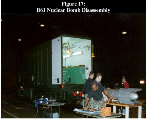
B61 maintenance with Weapons Maintenance Truck inside Protective Aircraft Shelter. A U.S. Air Force safety review determined in 1997 that there was a risk of accidental nuclear explosion during service of B61 nuclear bombs in NATO's protective aircraft shelters.
