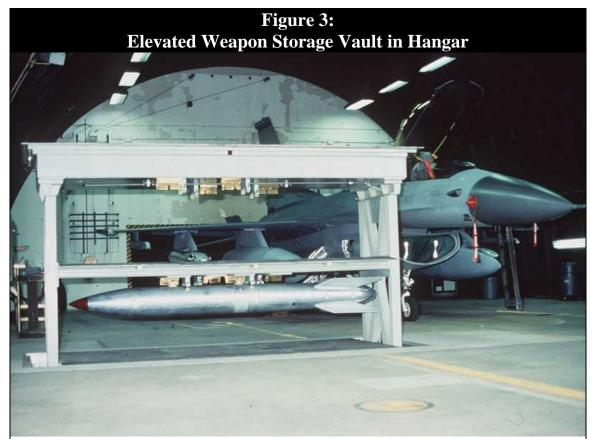
Elevated Weapons Storage Vault (WSV) with B61 body in Protective Aircraft Hangar with F-16 in the background. Notice the offset twin hangars in the ceiling of the top rack enabling storage of two offset weapons on each level for a total of four weapons in the vault. *Source: U.S. Air Force.*
