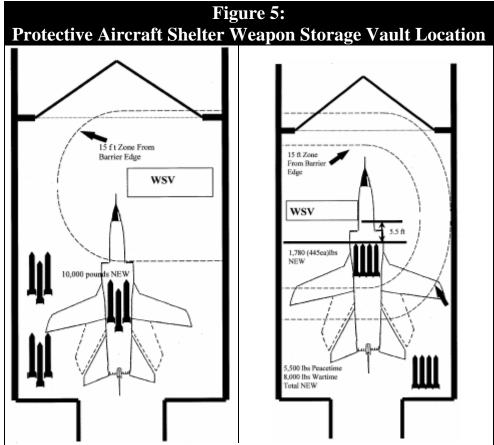
Two Protective Aircraft Shelter (PAS) configurations when conventional munitions are stored in the hangar with nuclear weapons in the underground Weapons Storage Vault (WSV): left – large shelters (37.5x23 meters) that permit 15-foot barrier from the WSV; right – small shelters (31.5x17 meters) that are too small to permit 15-foot barrier.
