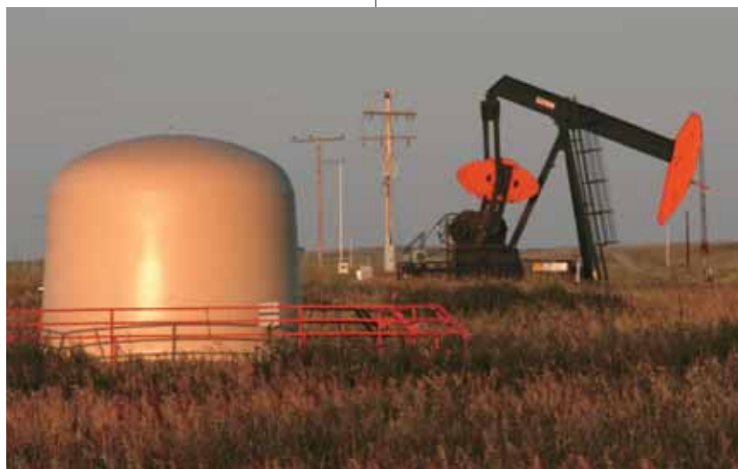
The plastic igloos on this Saskatchewan oil field house pipes that inject CO 2 into the ground to force out the very last drops of oil.
