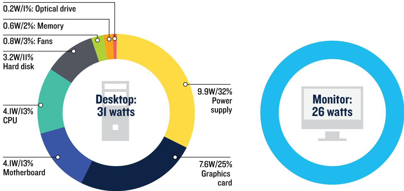
Figure 4 illustrates the power draw of the main components of a typical desktop computer in idle mode.
