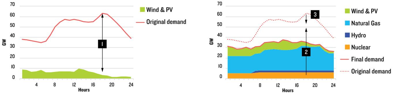
[1] Most challenging system conditions: 60 GW gap between demand and wind and solar output (Jan). [2] Nuclear, hydro and gas produce 32 GW of output. [3] Smart resources reduce generation needed by 28 GW.
