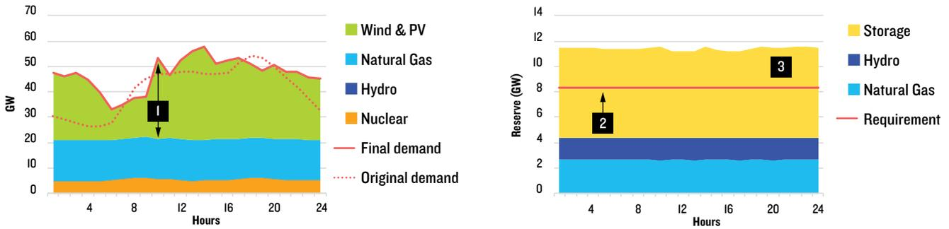
[1] Most challenging system conditions: 30 GW wind output (Apr). [2] During high wind conditions, 8 GW of reserves are needed. [3] Spare gas, hydro and storage exceed reserve needs.
