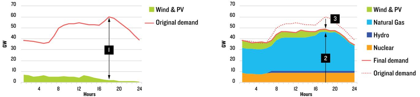
[1] Most challenging system conditions: 58 GW gap between demand and wind and solar output (Jan). [2] Nuclear, hydro and gas produce 47 GW of output. [3] Smart resources reduce generation needed by 11 GW.
