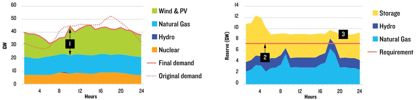
[1] Most challenging system conditions: 21 GW wind output (Apr). [2] During high wind conditions, over 7 GW of reserves are needed. [3] Spare gas, hydro and storage exceed reserve needs.
