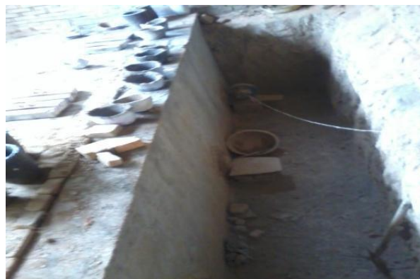
Figure 4. Pit-furnace of the family mill at Songcun village, July 2014.
