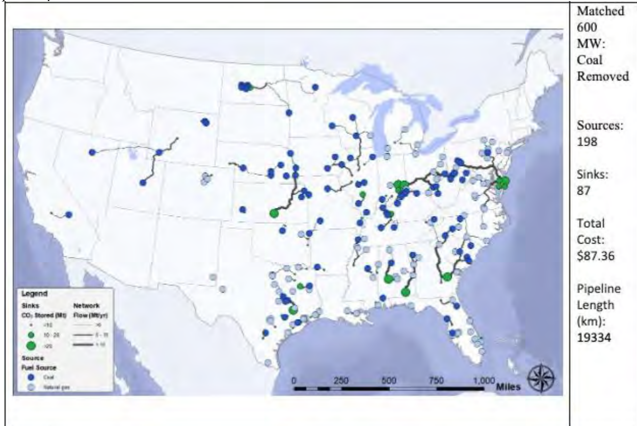
Figure 16. Infrastructure and costs associated with CCS at covered coal-fired and gas-fired power plants
