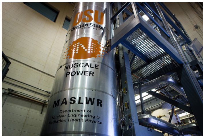
A one-third-scale model of a NuScale Power module at the company’s test facility.
