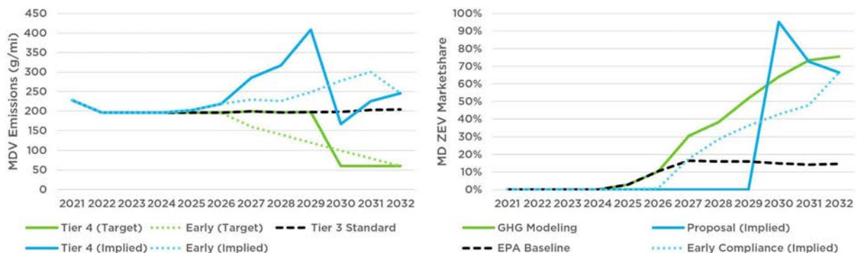
Figure VIII.B-2. Emissions performance and ZEV market share implied by the combination of achieving the proposed MDV GHG standards and MDV Tier 3 / Proposed Tier 4 NMOG+NOx standards
