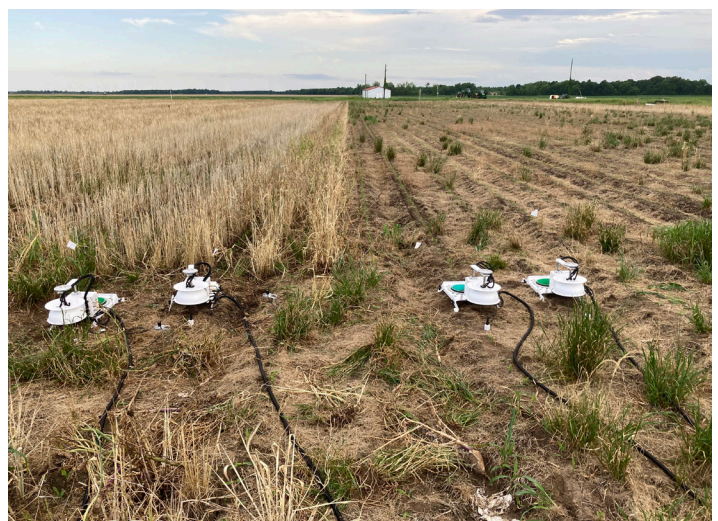
Instruments such as flux chambers are vital for tracking nitrous oxide emissions.
