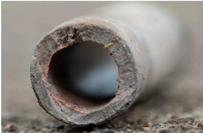
Part of a lead service line removed from outside a home in the West Roseland neighborhood of Chicago.
