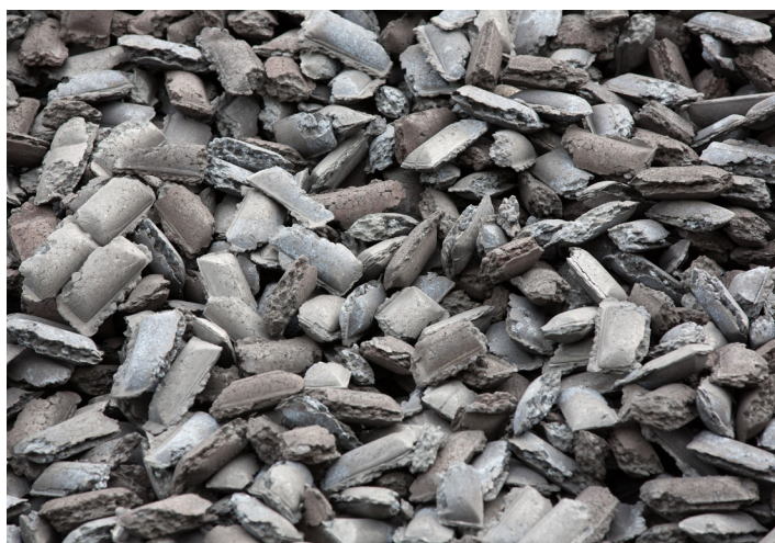
A pile of hot-briquetted iron, a form of DRI suitable for shipping.
