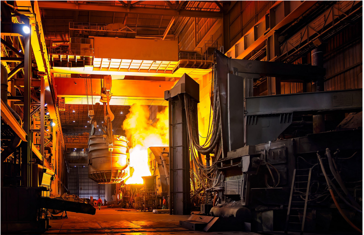
An electric arc furnace at the Steel Dynamics Columbus mill in Columbus, Mississippi.
