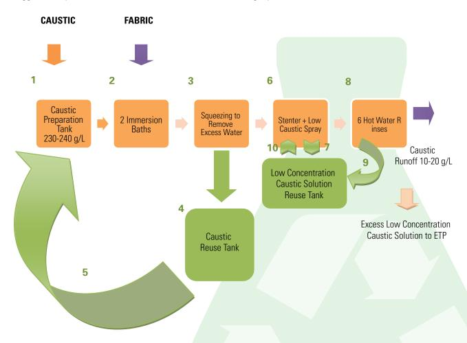
This amounts to savings of about Tk 0.18 to 0.27 per yard of fabric processed based on caustic soda usage on average of 90 grams per yard. The system costs between US \$400 and \$500 (Tk 30,000 to 40,000). To institute this process, a factory needs to invest in a corrosion-resistant pump and appropriate piping.
