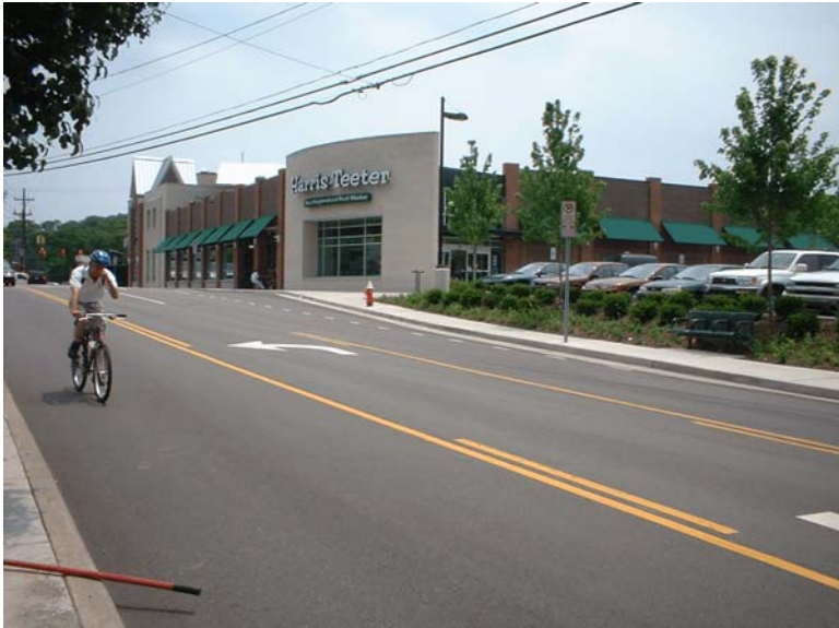
Commercial development serving the area from an adjacent neighborhood (note zero setback for pedestrian/transit orientation).
