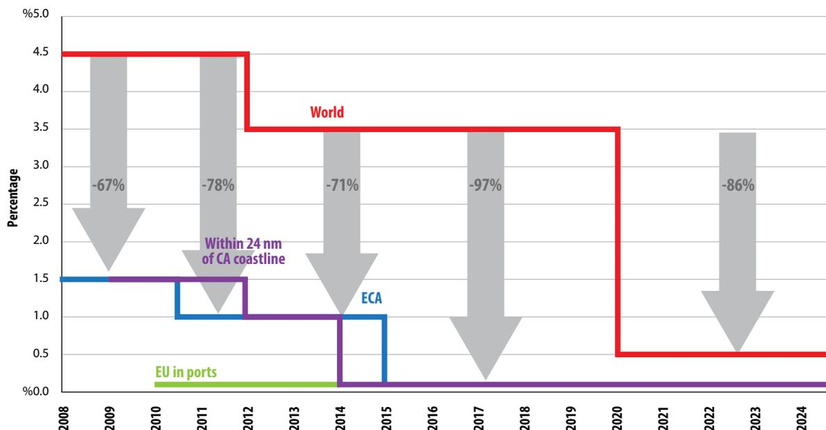
The above line for the California (CA) fuel sulfur standard shows the sulfur standards for marine gas oil (DMA); a stricter standard for marine diesel oil (DMB) requires a sulfur level not exceeding 0.5% beginning July 1, 2009, and 0.1% from January 1, 2014 onward. The Baltic Sea and the North Sea ECAs went into effect in 2006 and 2007 respectively. The North American ECA started implementation on August 1, 2012, the same day that the California 1% fuel sulfur requirement went into effect.
