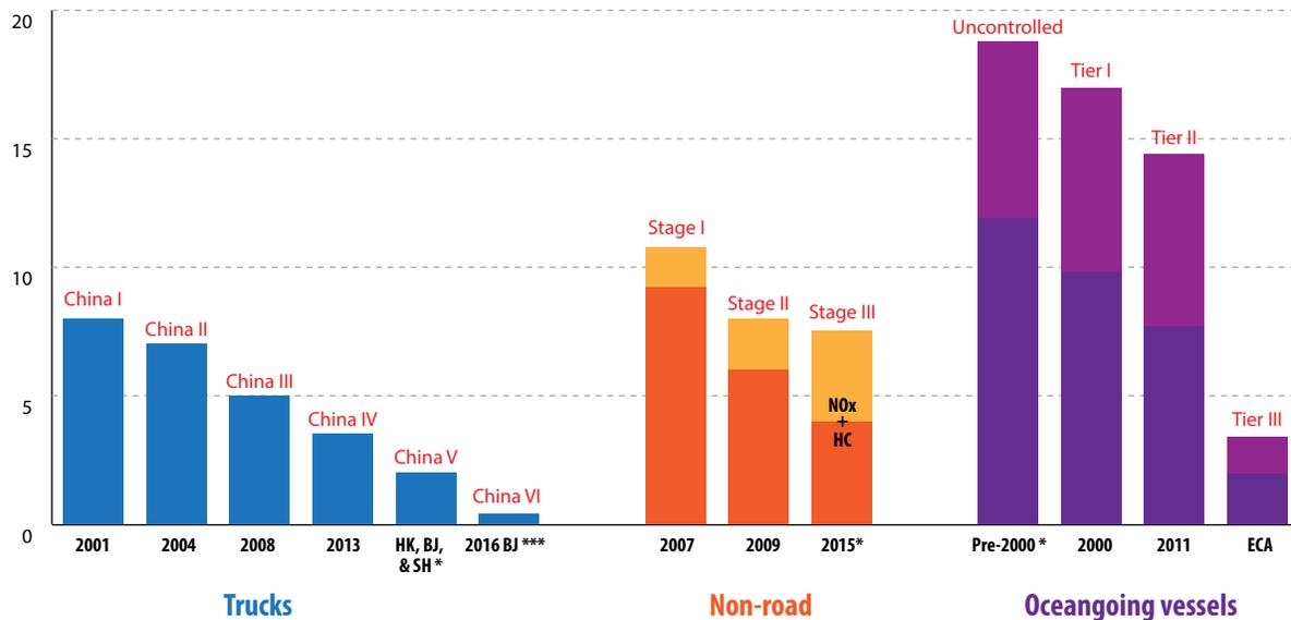
Where present, the lighter colors at the top of the bars indicate the range of NO<sub>x</sub> standards that vary by engine power or speed. The NO<sub>x</sub> standards for China non-road engines are set on the basis of power output, and the IMO NO<sub>x</sub> standards for OGVs vary by maximum engine speed. SH denotes Shanghai, HK denotes Hong Kong, and BJ denotes Beijing.
