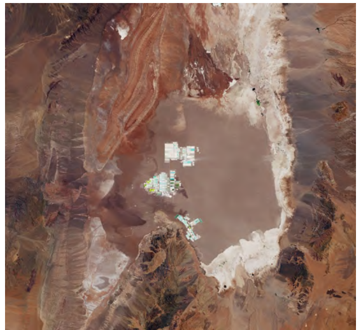
Solar evaporation ponds, like these in Chile’s Atacama Salt Flat, use huge amounts of brine pumped from beneath the salt flat to obtain lithium
