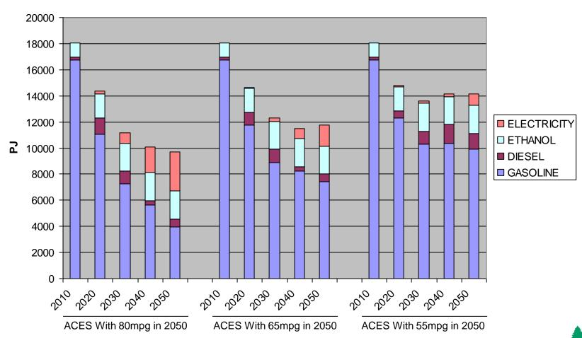
LIGHT-DUTY VEHICLES FUEL CONSUMPTION WITH DIFFERENT VEHICLE EFFICIENCY STANDARDS
