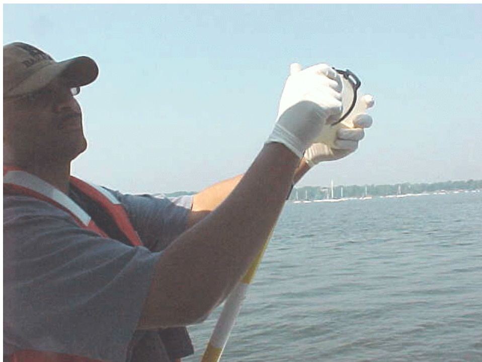
Photo 2: Attaching a sample bottle to a dipper handle in preparation for collecting a sample.
