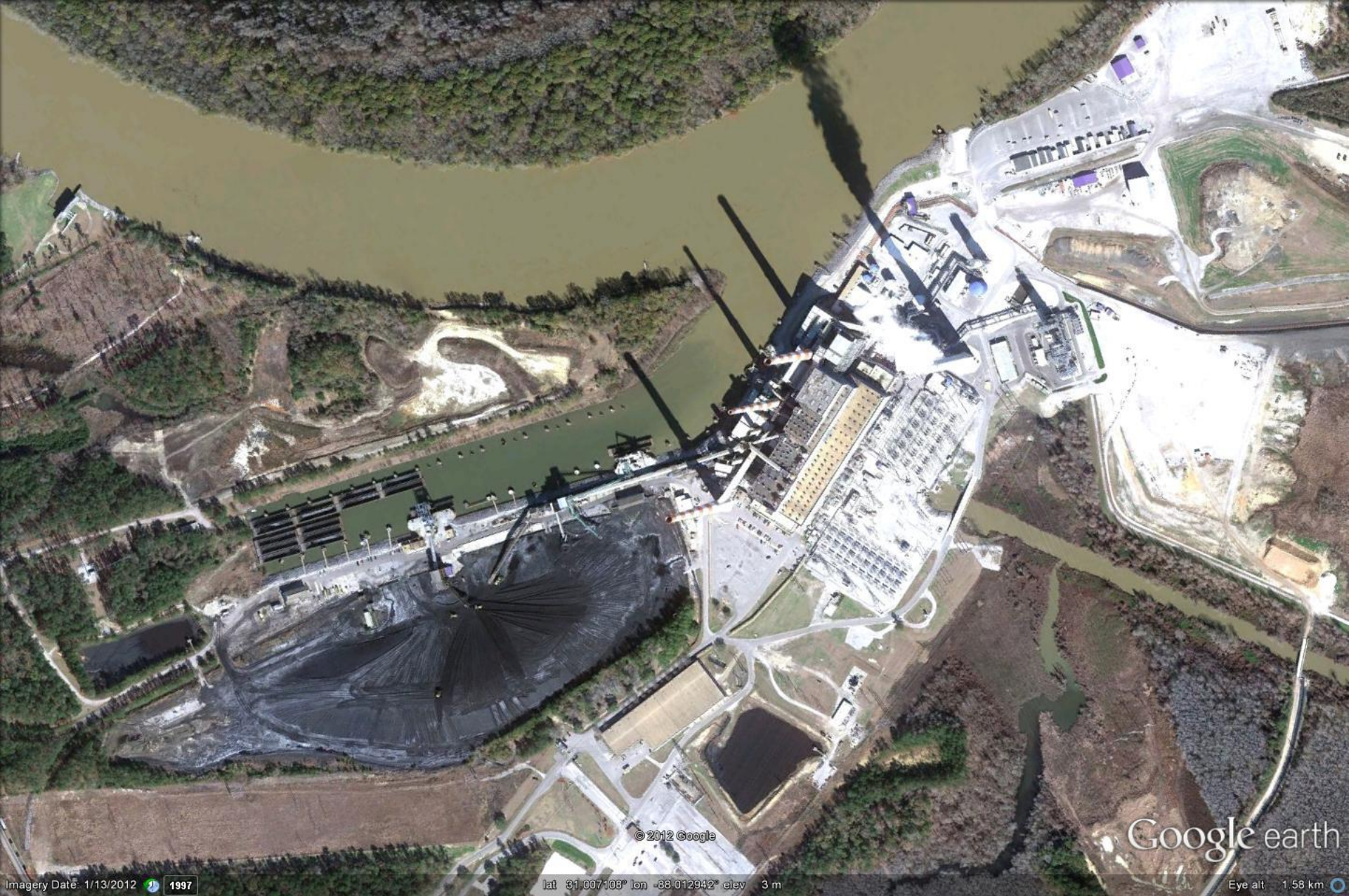
James M. Barry Electric Generating Plant (AL): five coal-fired units, which came online in 1954–1971, with respective generating capacities of 138 MW, 137 MW, 249 MW, 362 MW, and 750 MW. Five natural gas-fired units, including three combined cycle combustion turbines (173 MWe each of winter capacity) and two combined cycle steam turbines (193 MWe each of winter capacity), were installed in 2000.
