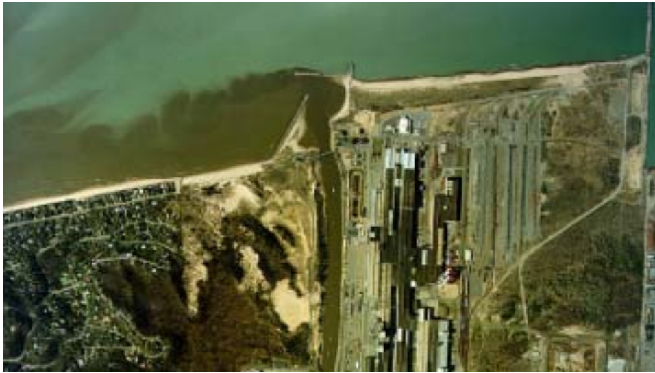
Figure 1 Sewage Contamination at Ogden Dunes Beach on Lake Michigan. Aerial photo of Burns Waterway, Porter County, Indiana, Earth Day, April 22, 2000, one day after a major rain storm and a 20 million to 30 million gallon combined sewer overflow reported by the City of Valparaiso. Photo: Lake Erie Land Company, Coffee Creek Watershed Conservancy Project, and Tom Anderson, Save the Dunes Council. 44
