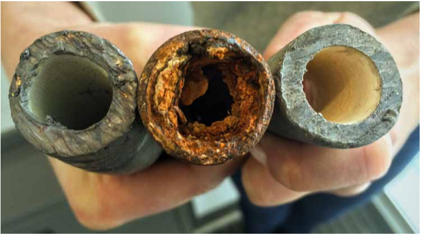
Pictured from left to right are a lead pipe, a corroded steel pipe, and a lead pipe treated with protective orthophosphate. Orthophosphate creates a film coating inside of lead pipes that can act as a barrier, reducing at least somewhat the amount of lead that gets into tap water.
